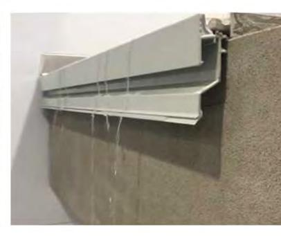
This profile is made of varnished aluminium. It is designed to protect the edges of tiles laid on terraces and balconies and to ensure proper water discharge. The profile is provided by a spacer that guarantees its correct positioning and by an open cell polyurethane adhesive strip that prevents silicone from blocking the drain holes.
